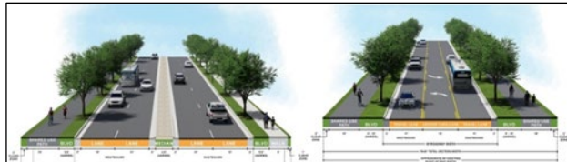
4-lane and 3-lane roadway configurations with pedestrian, bicycling and transit improvements are proposed and examined for Central Entrance.
